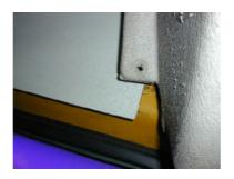
And lastly, re-attach the center molding that should cover both edges of the headliner where they meet in the middle. Tighten all screws after both sections of headliner is in place.
